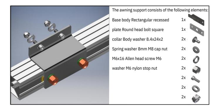
Please note that only the rectangular plate (with screws) must be inserted into the profile. The washer of body is mounted between the profile and the support.
