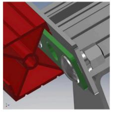
Insert the two side profiles (on each side of the vehicle) into each other and align the connecting plate in the middle.
